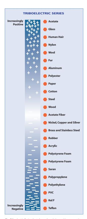
The Triboelectric Series chart shows the relative positive or negative charge of various materials.
