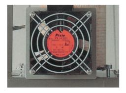
Use an external fan for faster response and more accurate measurement. It is in combination with this fan that the maximum capability of measurement for temperature and humidity can be achieved.
