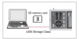
All measurement results are stored on an SD memory card. Data can be transferred by connecting a sound level meter to a Windows-based PC via a USB cable or an SD memory card directly into a PC card slot. The data inside of an SD memory card can be read on a Windows-based PC without any special software in either case. If required, spreadsheet or other similar software can be freely used to process the measured data.
