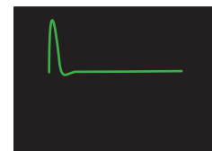
Second order impulse response (damping coefficient 0.7)
