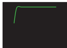
Second order step response (damping coefficient 0.7)
