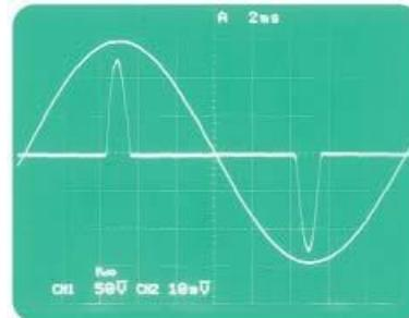
PCR-W/W2 Series output waveform (50 V/div, 5 A/div)
