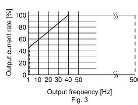
\* Output voltage rate: Percentage taking 100 V / 200 V (100 V / 200 V output range) as 100%.
