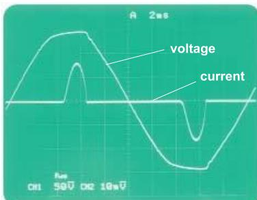
Commercial line output waveform (50 V/div, 5 A/div)
