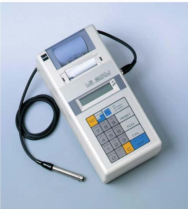
The LE-200J is a portable coating thickness tester with a built-in printer. This unit can accurately and quickly measures many items such as magnetic plating (electrolyzed nickel plating not included), coating, painting, and lining without injuring or damaging the item. Furthermore, you can print out the measurement results on-site with the internal printer.
