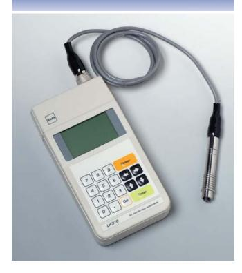
The LE-370 is a coating thickness tester capable of measuring the thickness of films such as electroplate (not including nickel electroplating) and paints coated onto ferrous metal substrates. It can transfer data to printers or PCs, and is also capable of simple statistical analysis, such as recording the number of measurements, average value, maximum and minimum values, and standard deviation.
