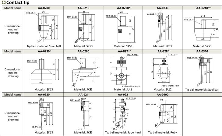
\*1 When affixing a flat gauge head such as the AA-0220/0240/0250 to a gauge with a measurement resolution of 1/1000 mm (1µm), adjustment of the degree of parallelization to match that of the surface of the measurement stand is required. In this case, the gauge head and stand must be purchased as a pair (additional cost required).
