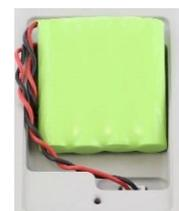
You can open the battery cover of DSV/DST, and replace it very easily.
